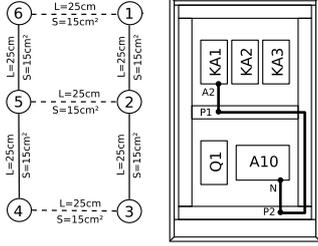
**Figure 3. Graph from Fig. 1 and routed cable**
