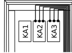
**Figure 4. Partial saturation of a conduit.**
